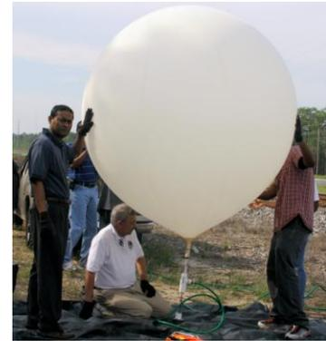
**Figure 12.** Filling the ASU balloon prior to launch.
